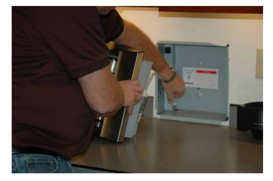
Step #2 Remove sprayhead by un-screwing counter clockwise.
